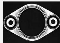
Stamping impact marks 30 parts/min
